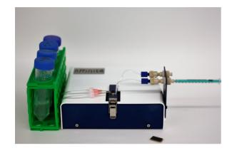
Label-free testing requires little to no preparation and, thanks to a compact design, can be performed at your bench. Simultaneous SPR analyses are conducted with three sample channels along with a reference channel.
